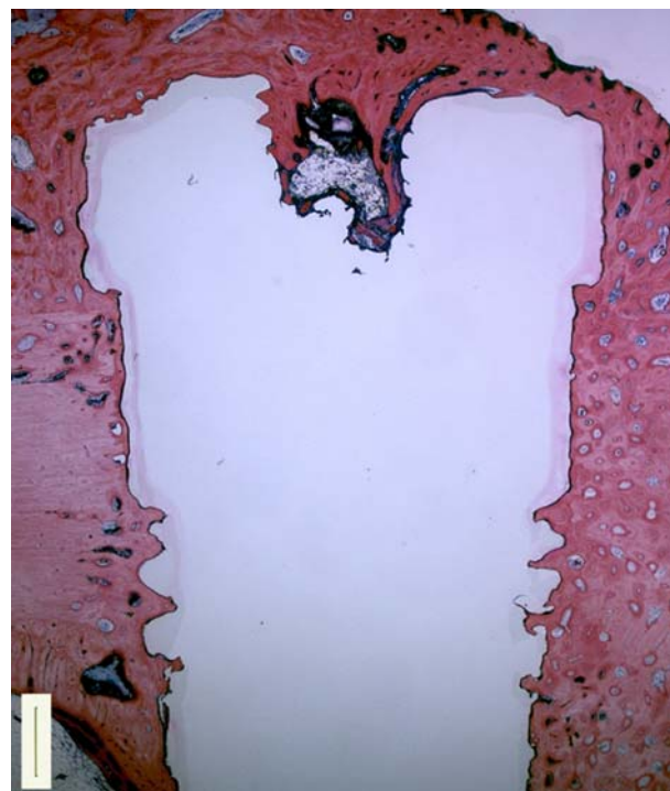
Fig. 3 Histological picture of a titanium coated PMMA implant. The implant is surrounded by bone tissue in close contact with the titanium coating, which is visible as a thin black line of the outer surface of the implant. Magnification 1.6 \times , bar = 625 \mu m
